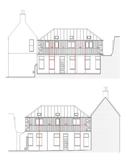
Images demonstrating the alignment of the new first floor windows with those existing at ground floor level.
